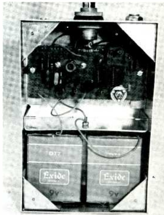
An internal view of the transmitter. This also shows the angled corner brackets, to which the back plate is secured
